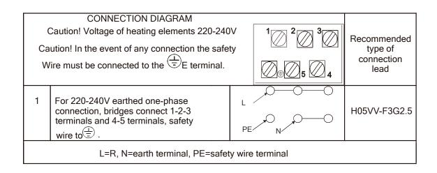
The connection cable must be secured in a strain-relief clamp.For the connection leads, the grounding wire must be longer than the other wires.
